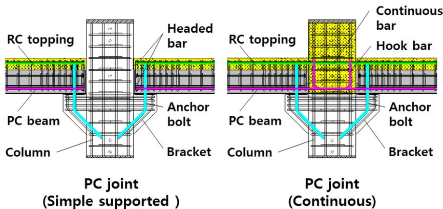
Fig. 1 Connection details of PC structures in Korea
