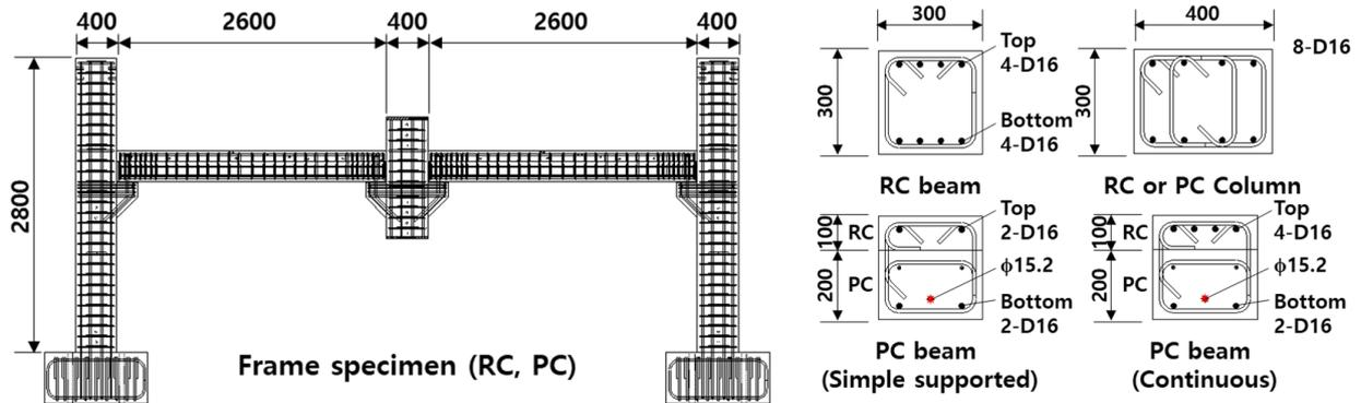
Fig.2 Details of the specimen
