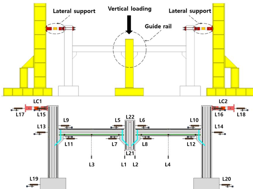
Fig.3 Test setup
